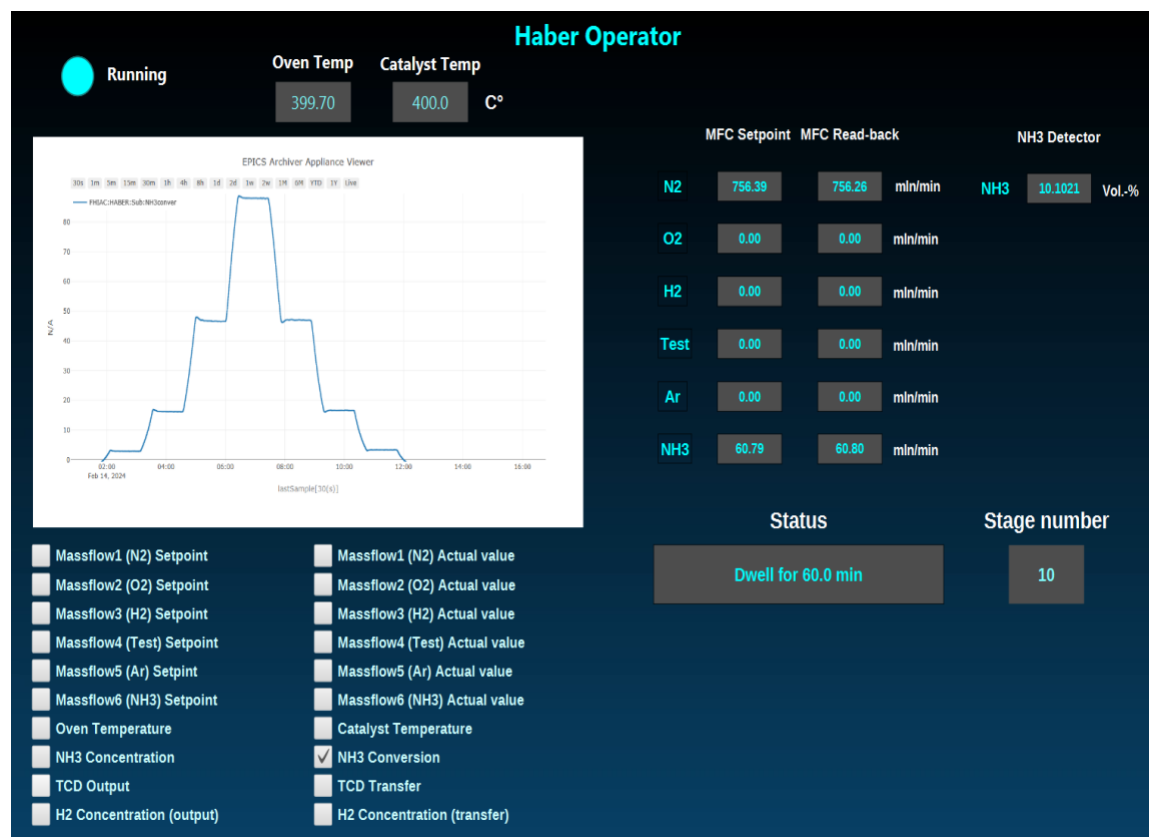
Fig. S4. The operator GUI is a read-only GUI for displaying historical and live plots as well as the status of the experiment and the read-back values from the devices.
