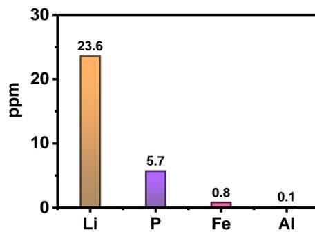
Figure S11 The concentrations of elements in the leachate (conditions: S/L (g/mL) ratio of 1:37.5, the mechanochemical time of 10 min, room temperature, and the rotational speed of 1000 rpm).
