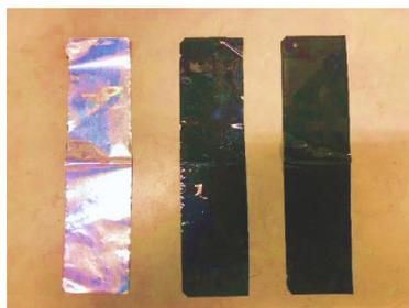
Figure S7 Physical image of cathode materials and aluminum foil after hydro-oxygen separation.
