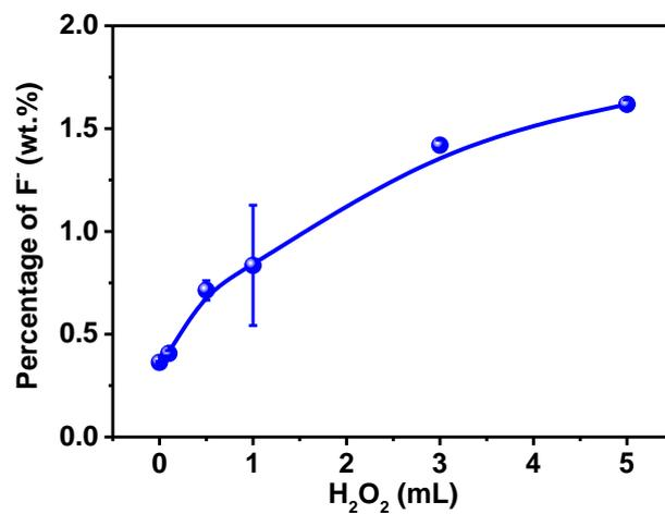
Figure S9 The leaching percentage of fluoride ions in hydro-oxygen solutions with different H<sub>2</sub>O<sub>2</sub> concentrations.
