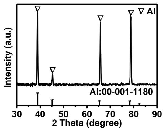
Figure S6 XRD patterns of the peeled aluminum foil products
