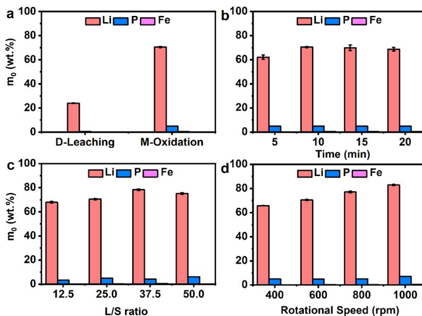
Figure S13 (a) the oxidative extraction efficiencies of Li in different scenarios (I) Direct leaching of cathode material piece; (II) Li extraction by mechanochemical oxidation (M-oxidation); different extraction parameters: (b) time, (c) S/L (g/mL) ratio, and (d) rotational speed, on Li extraction efficiencies.
