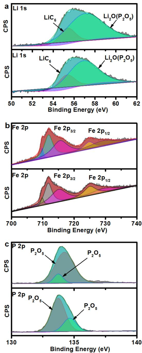
Figure S5 XPS high-resolution energy spectra of (a) Li 1s, (b) Fe 2p, (c) P 2p of CE (up) and LFP (down) cathode materials.
