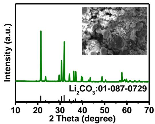
Figure S12 The XRD pattern and SEM image of the obtained  $\text{Li}_2\text{CO}_3$  product
