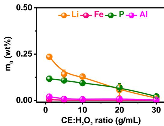
Figure S4 Effects of CE:H<sub>2</sub>O<sub>2</sub> ratio on the leaching percentages of elements during the hydro-oxygen separation (time of 0.25 min).
