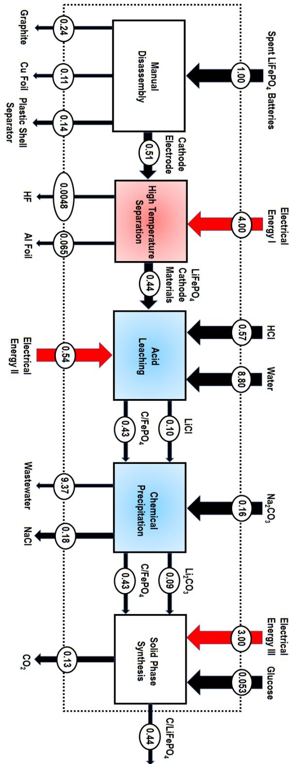
Figure S2 Life cycle boundaries for pyrometallurgy & hydrometallurgy route
