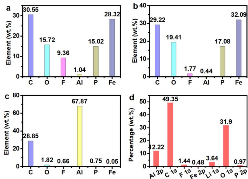
Figure S8 EDAX results of different products (a) cathode electrode, (b) cathode materials, (c) aluminum foil; (d) XPS results of aluminum foil.
