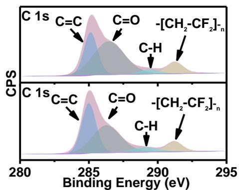
Figure S10 High-resolution C 1s spectra of cathode materials (a) before and (b) after hydro-oxygen separation.
