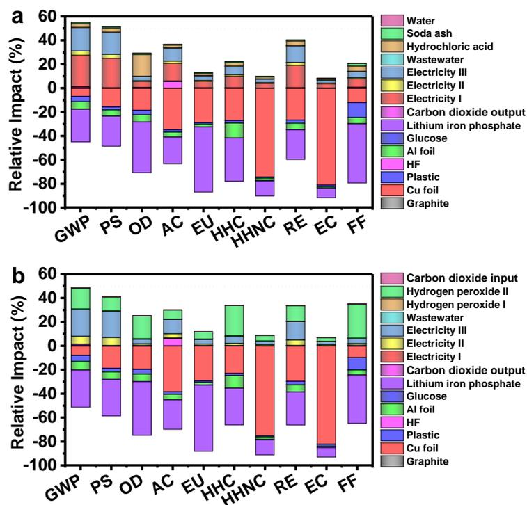
Figure S15 Contribution analysis of each material and energy consumption on the selected indicators: (a) pyro & hydro, and (b) HOR. Negative values indicate benefits (reduction of impacts due to recovered materials), positive values are environmental impacts (due to inputs for the recycling process).
