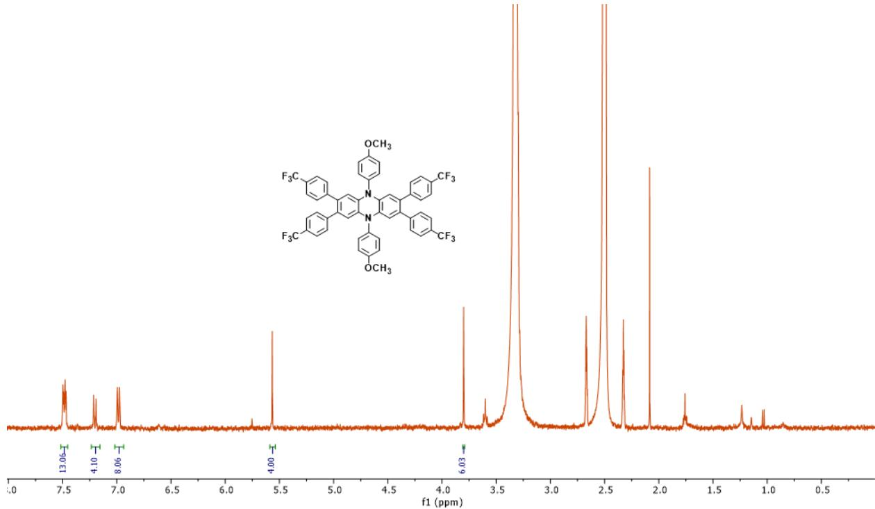
**Figure S117.**  $^1\text{H}$ -NMR spectrum of **4a** in  $\text{DMSO-d}_6$  after recrystallization.
