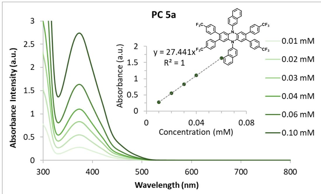
**Figure S7.** UV-Vis spectra of **5a** at varied concentrations in DMAc in a quartz cuvette with a pathlength of 1cm. Secondary graph demonstrates the Beer-Lambert law relationship between concentration and absorbance at 373 nm.
