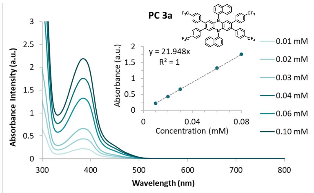
**Figure S4.** UV-Vis spectra of **3a** at varied concentrations in DMAc in a quartz cuvette with a pathlength of 1cm. Secondary graph demonstrates the Beer-Lambert law relationship between concentration and absorbance at 385 nm.
