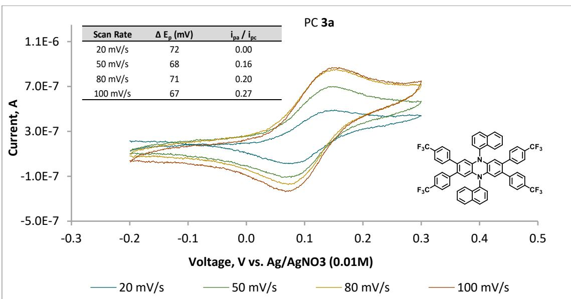
**Figure S55.** Cyclic voltammogram of PC 3a in DMAc at 20 mV/s, 50 mV/s, 80 mV/s, and 100 mV/s scan rates. Inserted into the graph is a chart showing the ratios of peak anodic current to peak cathodic current ( $i_{pa}/i_{pc}$ ) and the difference between peak anodic and peak cathodic current ( $\Delta E_p$ ) at each scan rate.
