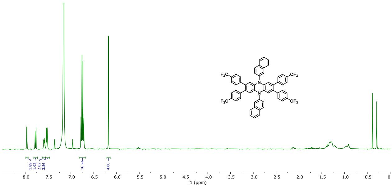
**Figure S121.**  $^1\text{H}$ -NMR spectrum of PC **5a** in  $\text{C}_6\text{D}_6$  after recrystallization.
