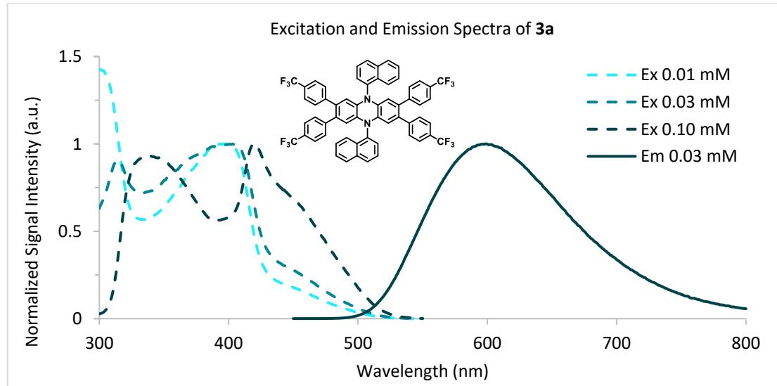
**Figure S9.** Fluorescence spectra of PC **3a**. Dashed lines are the excitation spectra at varying concentrations in DMAc and the solid line is the emission spectrum at 0.03 mM in DMAc. Emission spectra was collected using an excitation wavelength of 385 nm and is representative of emission profiles at all concentrations between 0.01 mM and 0.10 mM. Excitation spectra were collected for emission at 586 nm.
