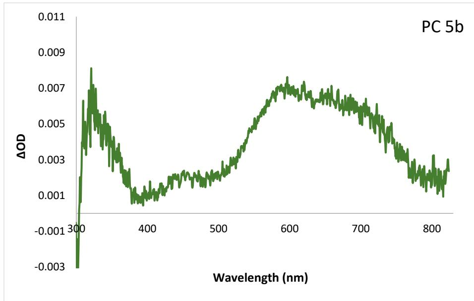
**Figure S27.** Spectral absorption of PC 5b in DMAc at a 200 ns time delay, with no emission subtraction. The ESA feature visible at  $\lambda = 550$  nm was followed by kinetic absorption. The spectral absorption data was offset corrected using kinetic data acquired at  $\lambda = 550$  nm.
