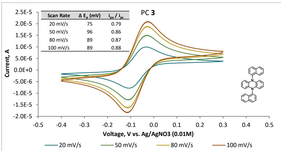
**Figure S54.** Cyclic voltammogram of PC 3 in DMAc at 20 mV/s, 50 mV/s, 80 mV/s, and 100 mV/s scan rates. Inserted into the graph is a chart showing the ratios of peak anodic current to peak cathodic current ( $i_{pa}/i_{pc}$ ) and the difference between peak anodic and peak cathodic current ( $\Delta E_p$ ) at each scan rate.
