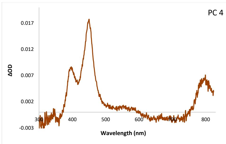
**Figure S22.** Spectral absorption of PC 4 in DMAc at a 400 ns time delay, with no emission subtraction. The ESA feature visible at  $\lambda = 450$  nm was followed by kinetic absorption. The spectral absorption data was offset corrected using kinetic data acquired at  $\lambda = 450$  nm.
