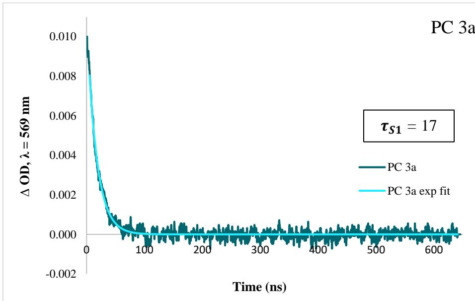
**Figure S29.** Kinetic emission trace for PC 3a in DMAc at 569 nm with an exponential tail fit for determination of  $\tau_{\text{S}1}$ .
