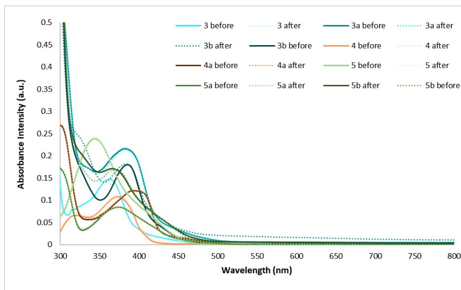
**Figure S45.** Overlaid UV-vis spectra of PC solutions used for TA spectroscopy, taken before and after TA spectroscopy was performed to monitor if PC degradation occurred. The PC solutions analyzed in this work did not show evidence of degradation after TA, indicated by no significant observable change in the UV-vis spectra before and after TA spectroscopy was performed.
