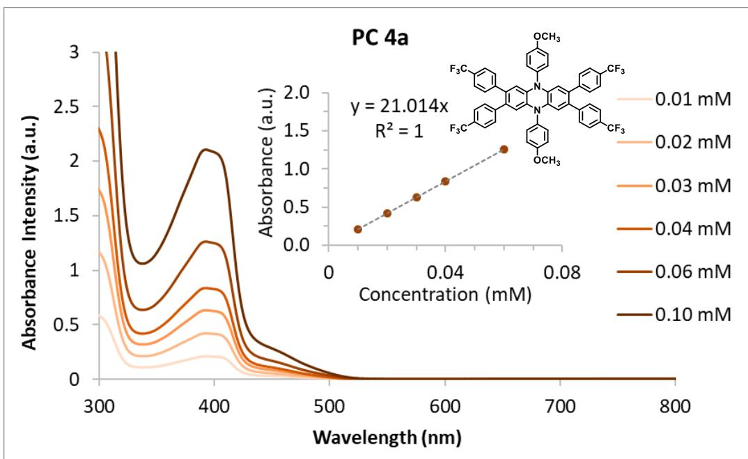
**Figure S6.** UV-Vis spectra of **4a** at varied concentrations in DMAc in a quartz cuvette with a pathlength of 1cm. Secondary graph demonstrates the Beer-Lambert law relationship between concentration and absorbance at 392 nm.
