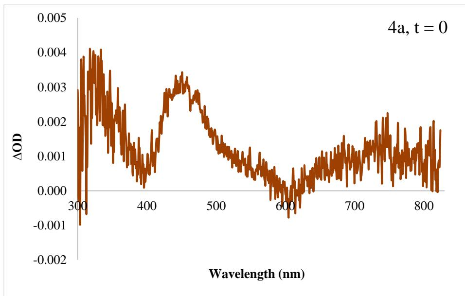
**Figure S24.** Spectral absorption of PC 4a in DMAc with a 0 ns time delay and with emission subtraction. The ESA feature at  $\lambda = 450$  nm was followed by kinetic absorption and fit with an exponential tail fit, resulting in determination of  $\tau_{S1} = 14$  ns, in agreement with  $\tau_{S1}$  determined by kinetic emission (13 ns). The spectral absorption data was offset corrected using kinetic data acquired at  $\lambda = 450$  nm.
