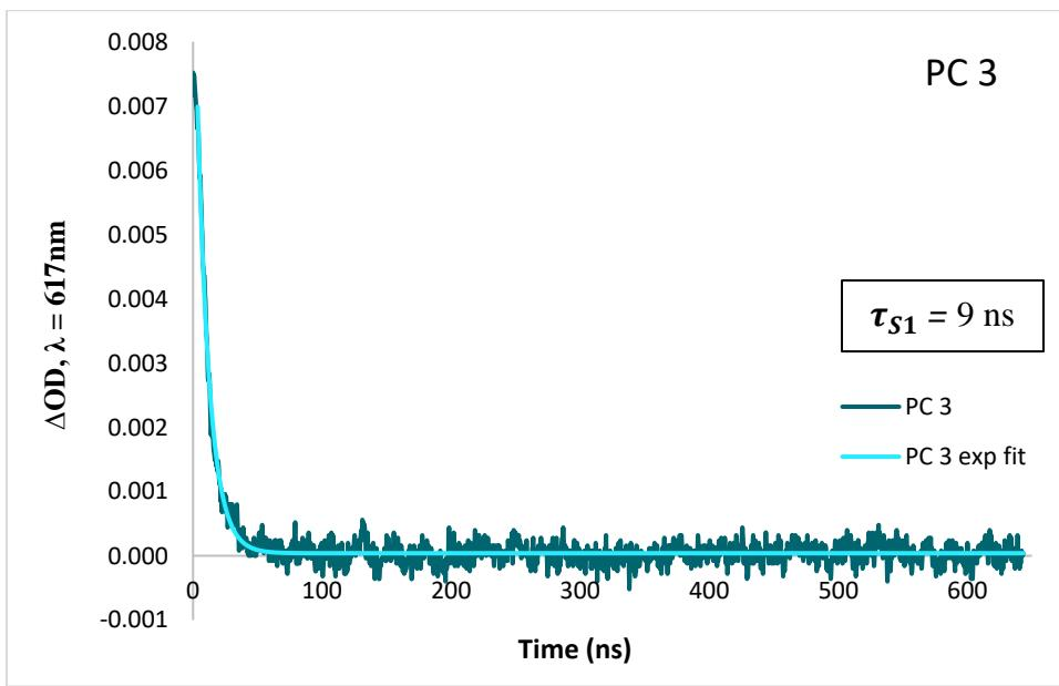
**Figure S28.** Kinetic emission trace for PC 3 in DMAc at 617 nm with an exponential tail fit for determination of  $\tau_{\text{S}1}$ .
