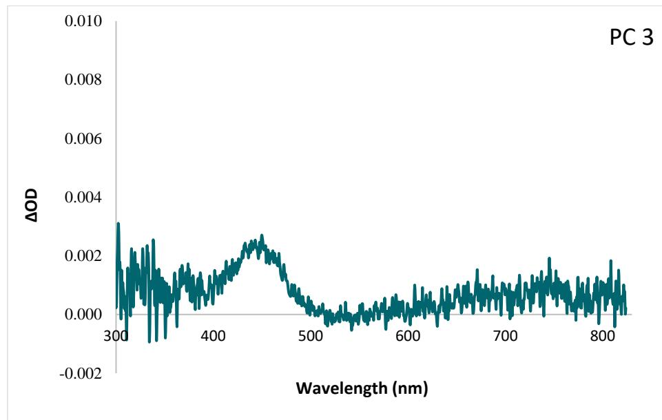
**Figure S19.** Spectral absorption of PC 3 in DMAc at a 200 ns time delay, with no emission subtraction. The excited state absorption (ESA) feature visible at  $\lambda = 445$  nm was followed by kinetic absorption. The spectral absorption data was offset corrected using kinetic data acquired at  $\lambda = 445$  nm.
