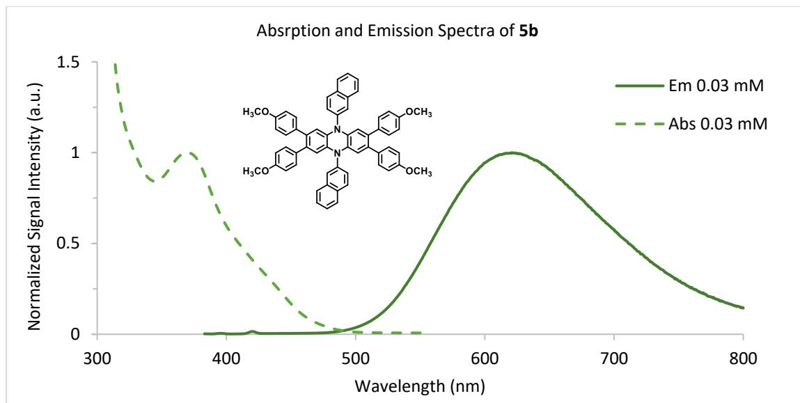
**Figure S18.** Emission spectra of PC **5b** (solid) and absorption spectra of **5b** (dashed) at 0.03 mM in DMAc. Absorption spectra was measured using UV-Vis and emission spectra was measured using fluorimetry. Emission spectra was collected using an excitation wavelength of 371 nm.
