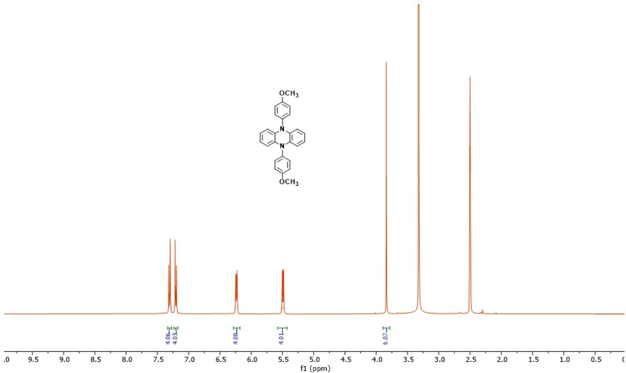
**Figure S114.** <sup>1</sup>H-NMR spectrum of PC 4 recrystallization from toluene-hexanes DMSO-d<sub>6</sub>.
