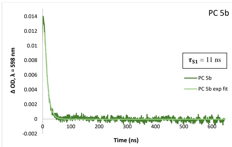
**Figure S35.** Kinetic emission trace for PC 5b in DMAc at 598 nm with an exponential tail fit for determination of  $\tau_{S1}$ . Kinetic emission was also measured at 457 nm, but  $\tau_{S1}$  was found to be less than the 6 ns duration of the instrument laser pulse (below limit of detection).
