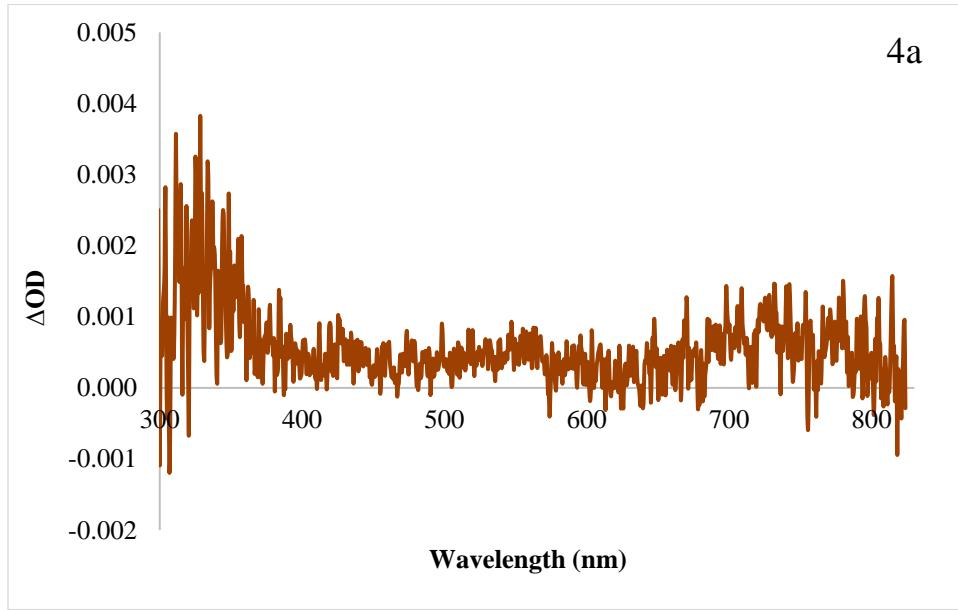
**Figure S23.** Spectral absorption of PC 4a in DMAc at a 200 ns time delay, with no emission subtraction. There are no distinguishable features that can be followed by kinetic absorption. The spectral absorption data was offset corrected using kinetic data acquired at  $\lambda = 450$  nm.
