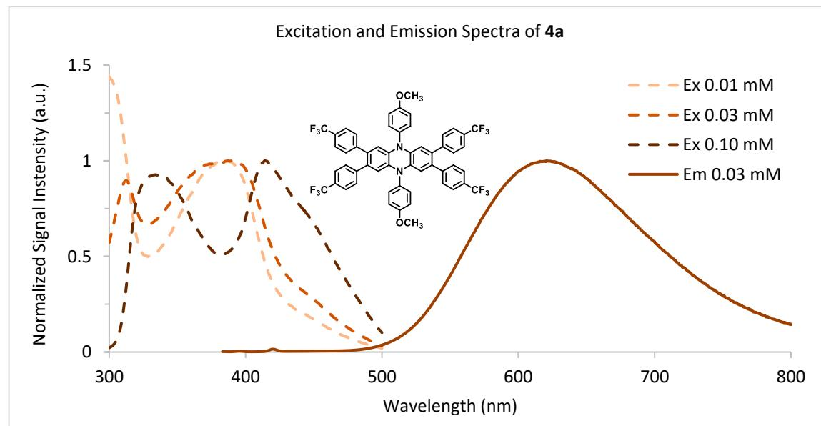
**Figure S13.** Fluorescence spectra of PC **4a**. Dashed lines are the excitation spectra at varying concentrations in DMAc and the solid line is the emission spectrum at 0.03 mM in DMAc. Emission spectra was collected using an excitation wavelength of 392 nm and is representative of emission profiles at all concentrations between 0.01 mM and 0.10 mM. Excitation spectra were collected for emission at 599 nm.
