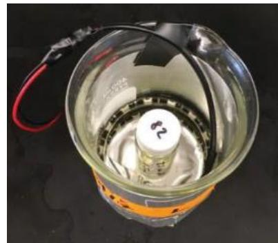
**Figure S1.** 400 mL white light LED beaker photoreactor for polymerizations.
