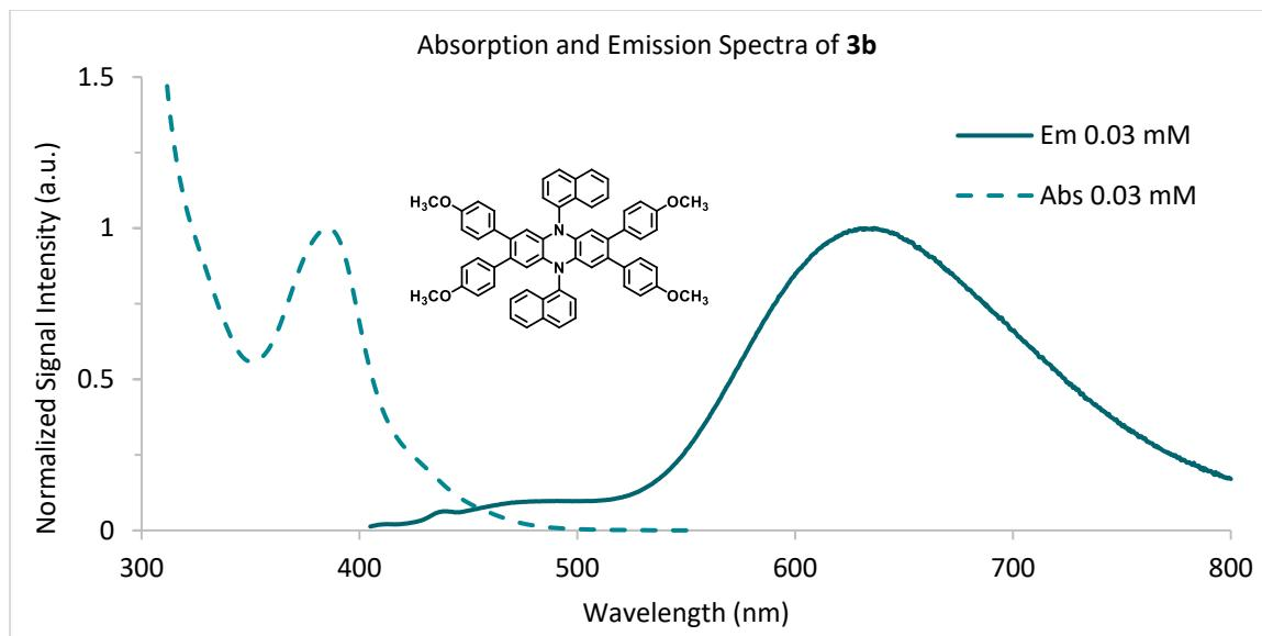
**Figure S12.** Emission spectra of PC **3b** (solid) and absorption spectra of **3b** (dashed) at 0.03 mM in DMAc. Absorption spectra was measured using UV-Vis and emission spectra was measured using fluorimetry. Emission spectra was collected using an excitation wavelength of 385 nm.
