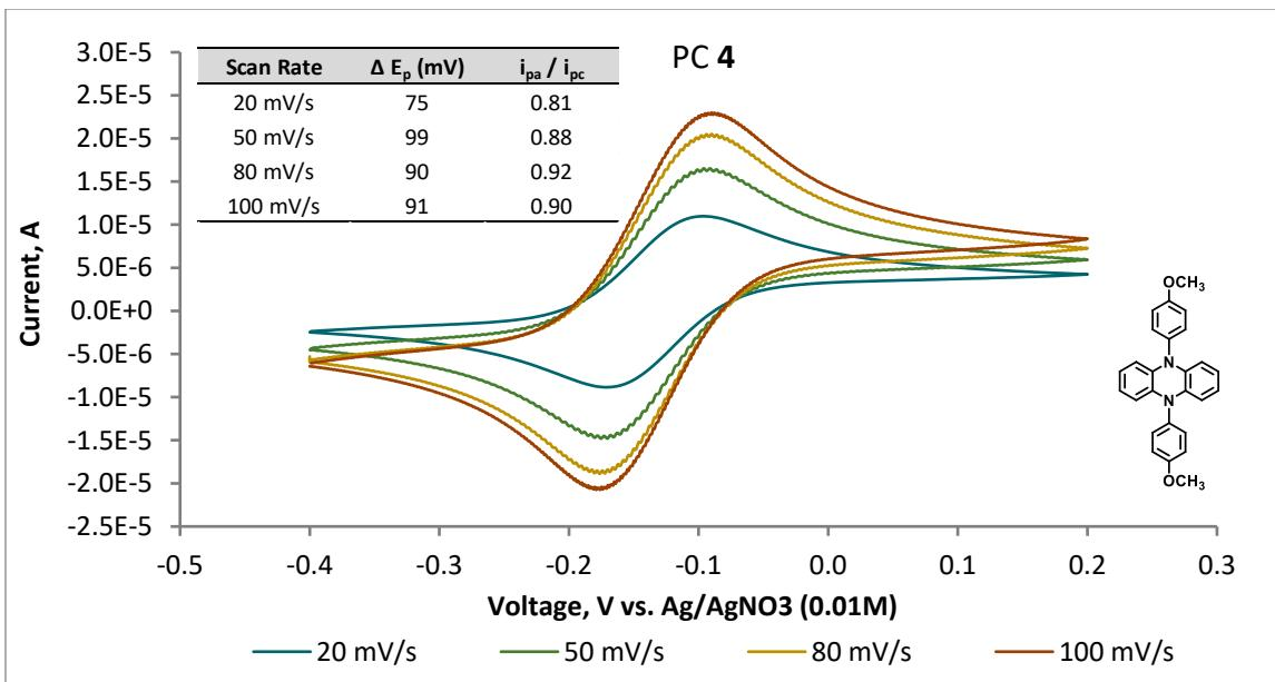
**Figure S57.** Cyclic voltammogram of PC 4 in DMAc at 20 mV/s, 50 mV/s, 80 mV/s, and 100 mV/s scan rates. Inserted into the graph is a chart showing the ratios of peak anodic current to peak cathodic current ( $i_{pa}/i_{pc}$ ) and the difference between peak anodic and peak cathodic current ( $\Delta E_p$ ) at each scan rate.
