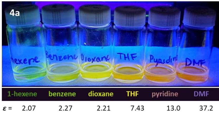
**Figure S50.** Photograph of PC 4a dissolved in solvents of increasing polarity (from left to right) while under irradiation with 365 nm light.
