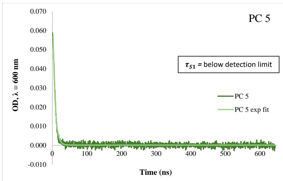
**Figure S33.** Kinetic emission trace for PC 5 in DMAc at 600 nm with an exponential tail fit for determination of  $\tau_{S1}$  is shown above, however  $\tau_{S1}$  was not reported because it was found to be less than the 6 ns duration of the instrument laser pulse (below limit of detection).
