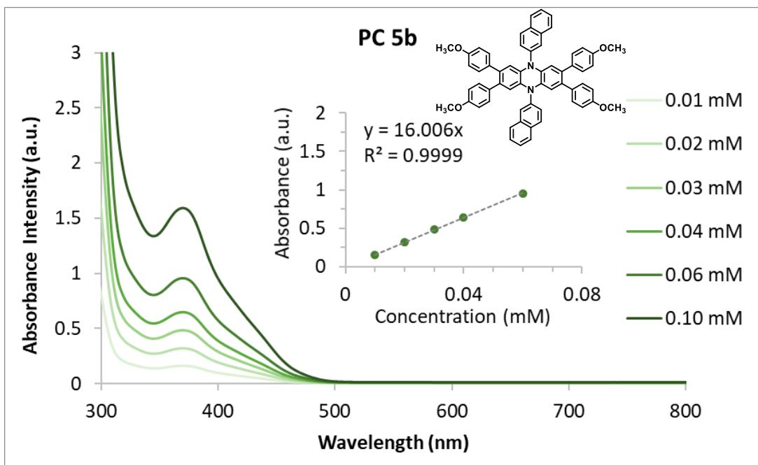
**Figure S8.** UV-Vis spectra of **5b** at varied concentrations in DMAc in a quartz cuvette with a pathlength of 1cm. Secondary graph demonstrates the Beer-Lambert law relationship between concentration and absorbance at 371 nm.
