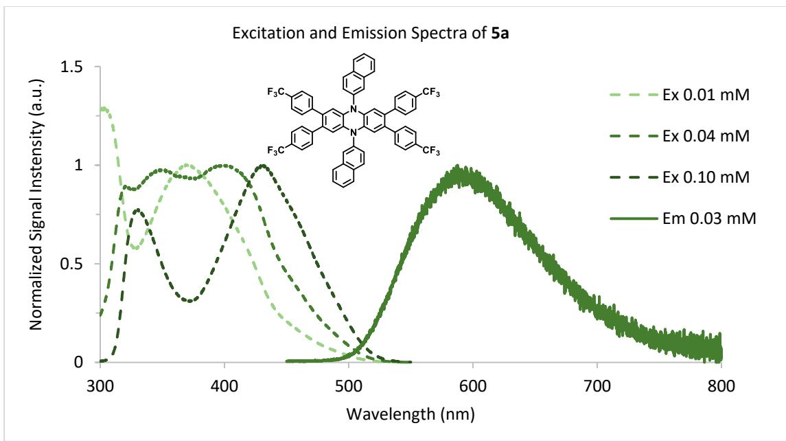
**Figure S15.** Fluorescence spectra of PC **5a**. Dashed lines are the excitation spectra at varying concentrations in DMAc and the solid line is the emission spectrum at 0.03 mM in DMAc. Emission spectra was collected using an excitation wavelength of 373 nm and is representative of emission profiles at all concentrations between 0.01 mM and 0.10 mM. Excitation spectra were collected for emission at 587 nm.
