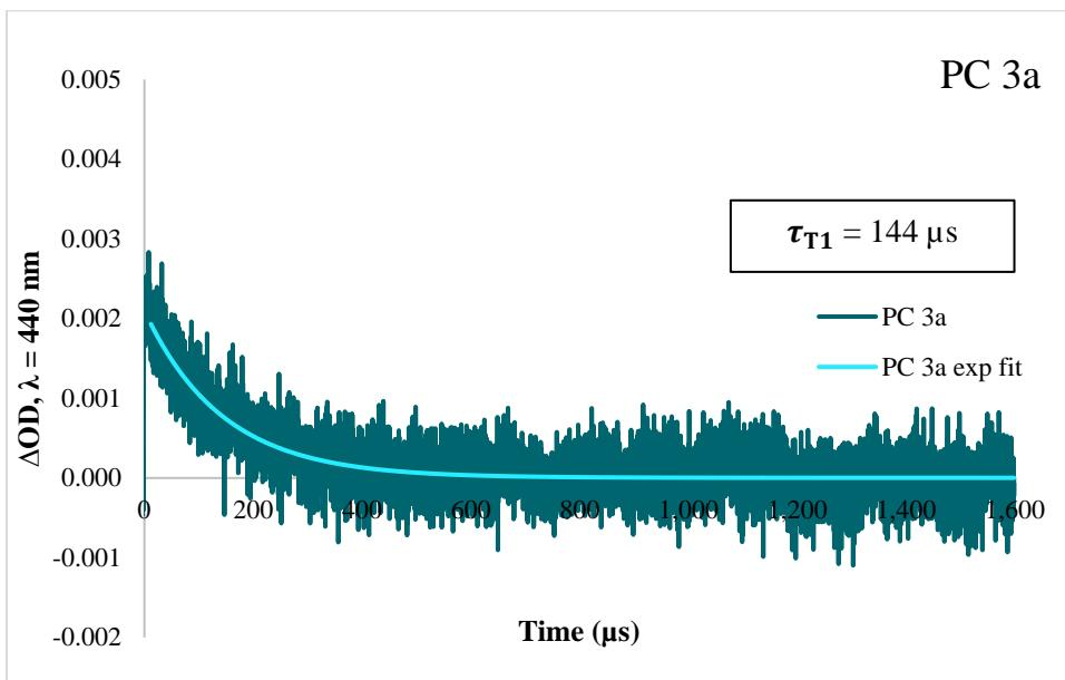
**Figure S37.** Kinetic absorption trace for PC 3a in DMAc at 440 nm with an exponential tail fit for determination of  $\tau_{\text{T1}}$ .
