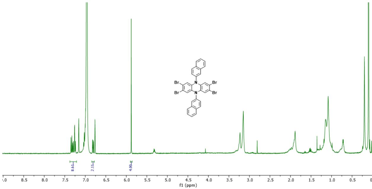
**Figure S120.**  $^1\text{H}$ -NMR spectrum of unpurified **5-4Br** in  $\text{C}_6\text{D}_6$ .
