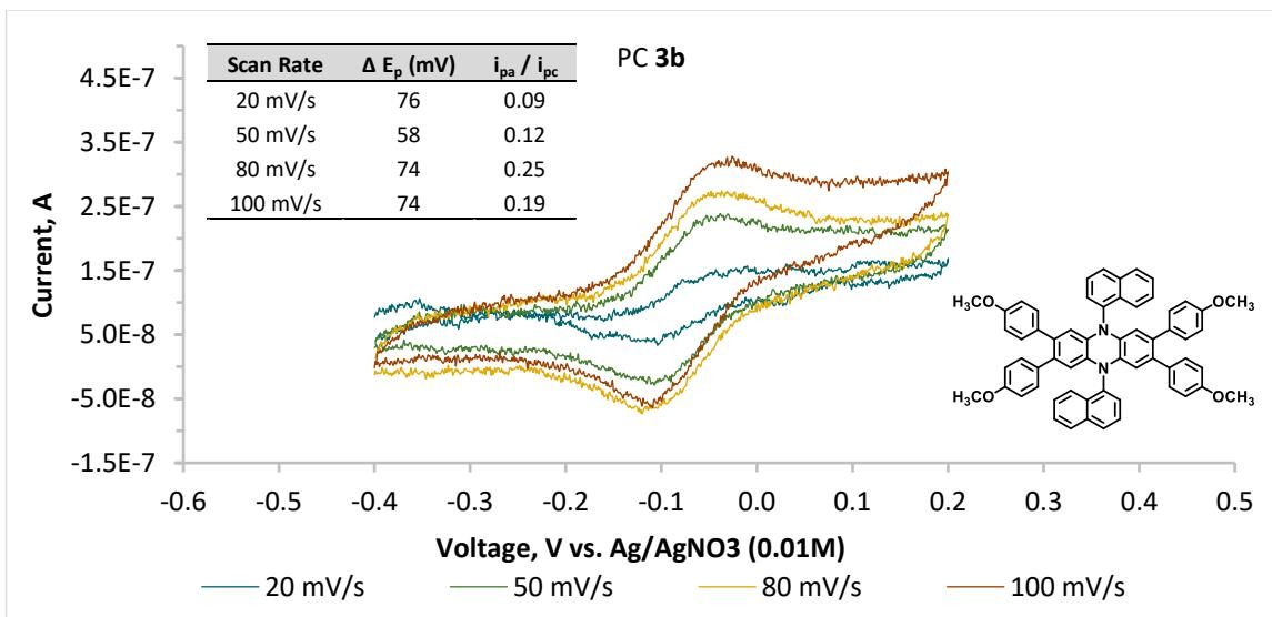
**Figure S56.** Cyclic voltammogram of PC 3b in DMAc at 20 mV/s, 50 mV/s, 80 mV/s, and 100 mV/s scan rates. Inserted into the graph is a chart showing the ratios of peak anodic current to peak cathodic current ( $i_{pa}/i_{pc}$ ) and the difference between peak anodic and peak cathodic current ( $\Delta E_p$ ) at each scan rate.
