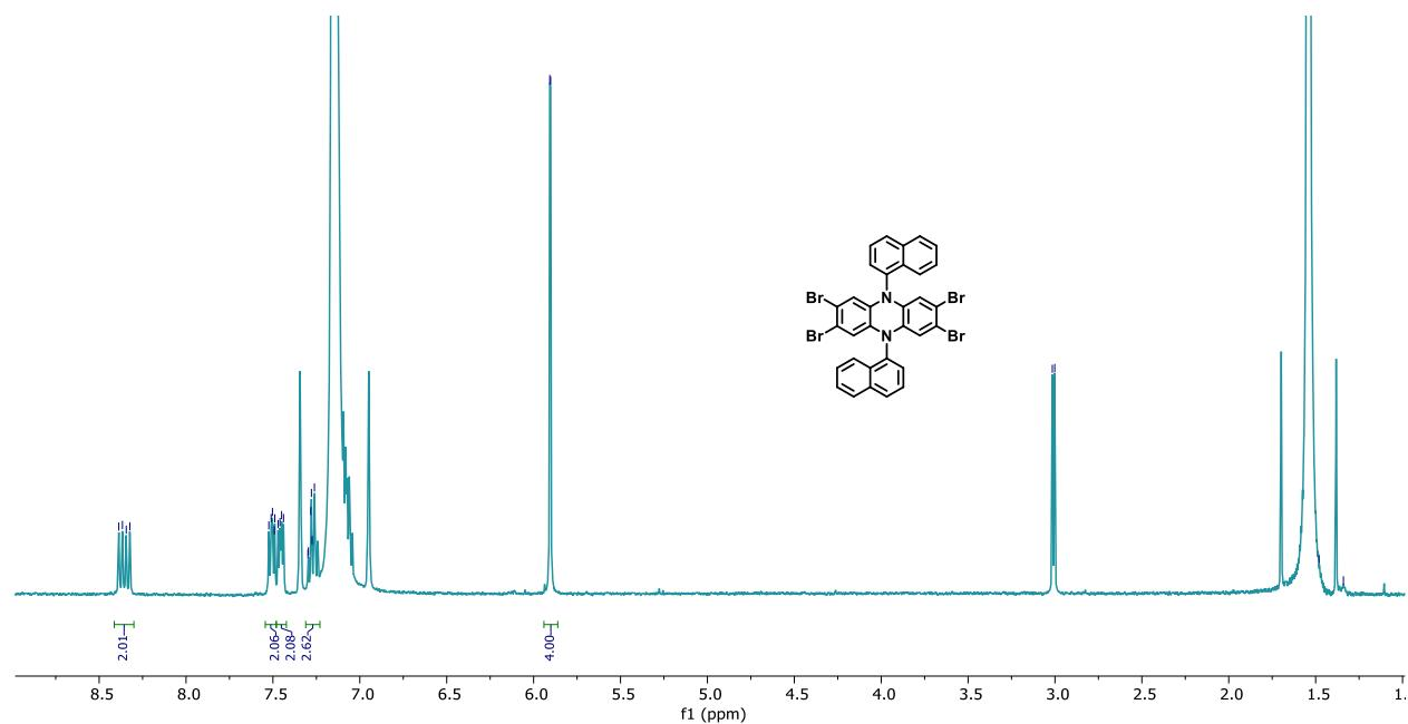
**Figure S110.** <sup>1</sup>H-NMR spectrum of unpurified PC 3-4Br in C<sub>6</sub>D<sub>6</sub>.
