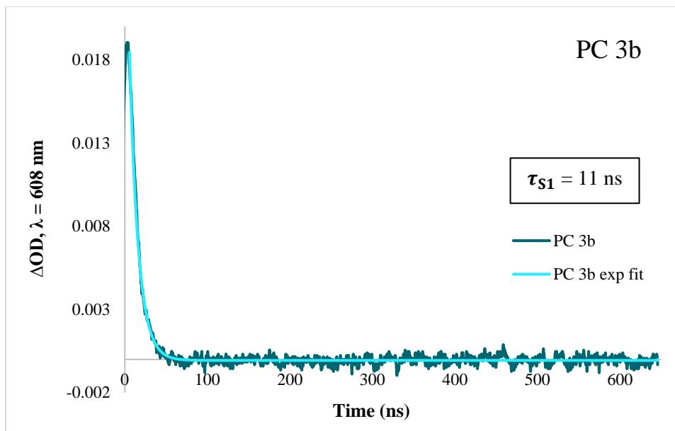
**Figure S30.** Kinetic emission trace for PC 3b in DMAc at 608 nm with an exponential tail fit for determination of  $\tau_{S1}$ . Kinetic emission was also measured at 462 nm, but  $\tau_{S1}$  was found to be less than the 6 ns duration of the instrument laser pulse (below limit of detection).
