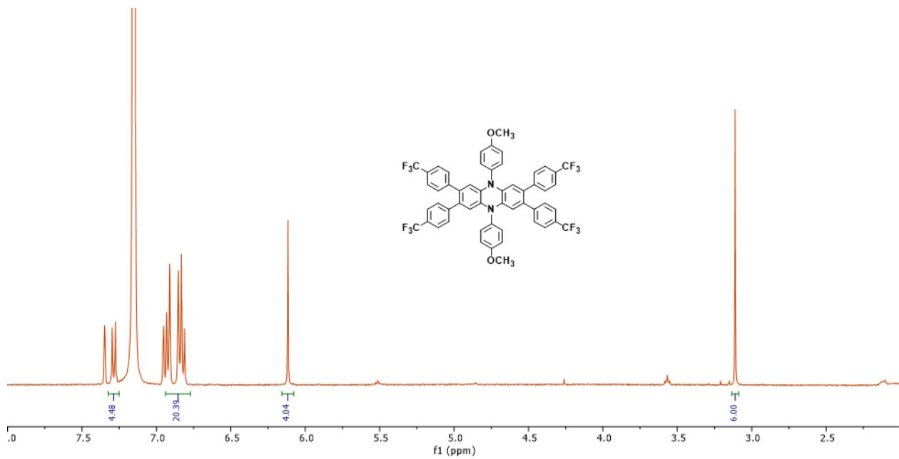
**Figure S116.**  $^1\text{H}$ -NMR spectrum of 4a in  $\text{C}_6\text{D}_6$  after recrystallization.
