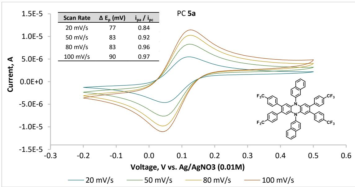
**Figure S59.** Cyclic voltammogram of PC 5a in DMAc at 20 mV/s, 50 mV/s, 80 mV/s, and 100 mV/s scan rates. Inserted into the graph is a chart showing the ratios of peak anodic current to peak cathodic current ( $i_{pa}/i_{pc}$ ) and the difference between peak anodic and peak cathodic current ( $\Delta E_p$ ) at each scan rate.
