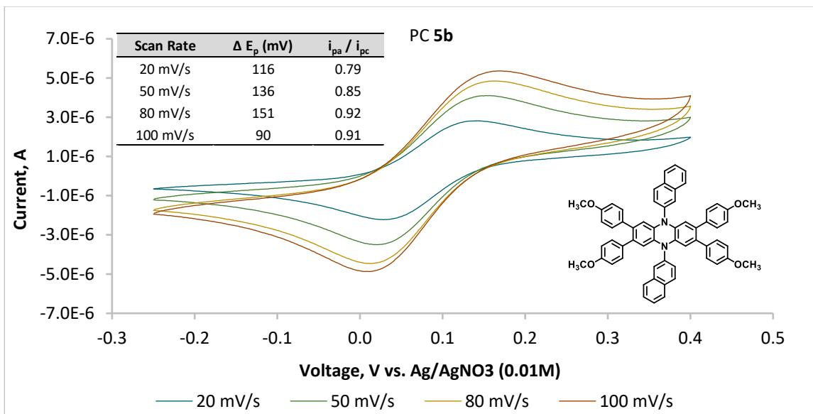
**Figure S60.** Cyclic voltammogram of PC **5b** in DMAc at 20 mV/s, 50 mV/s, 80 mV/s, and 100 mV/s scan rates. Inserted into the graph is a chart showing the ratios of peak anodic current to peak cathodic current ( $i_{pa}/i_{pc}$ ) and the difference between peak anodic and peak cathodic current ( $\Delta E_p$ ) at each scan rate.
