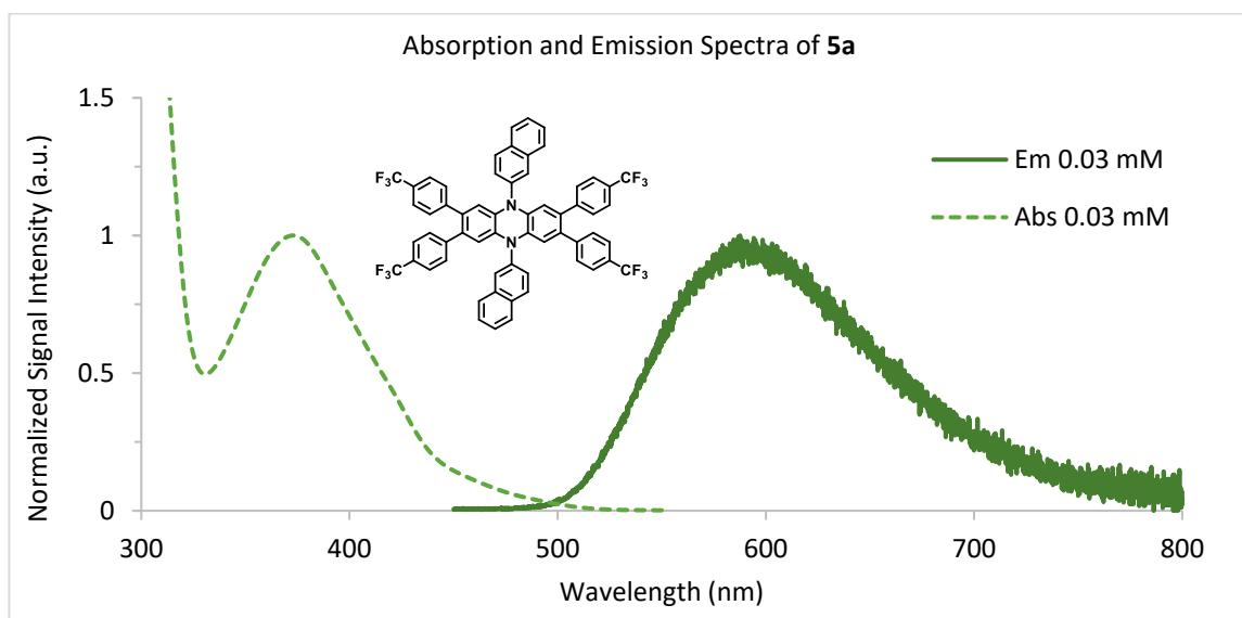
**Figure S16.** Emission spectra of PC **5a** (solid) and absorption spectra of **5a** (dashed) at 0.03 mM in DMAc. Absorption spectra was measured using UV-Vis and emission spectra was measured using fluorimetry. Emission spectra was collected using an excitation wavelength of 373 nm.
