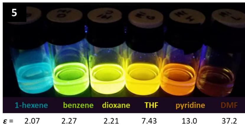
**Figure S51.** Previously reported Photograph of PC 5 dissolved in solvents of increasing polarity (from left to right) while under irradiation with 365 nm light. (*J. Am. Chem. Soc.* **2017**, *139*, 348–355)
