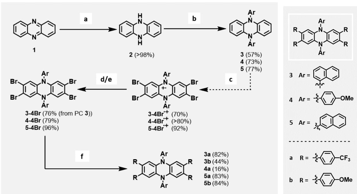
**Figure S3.** Synthetic scheme for synthesis of core-extended N,N-diaryl dihydrophenazines and structures. The mol percent yield from each step is noted adjacent to the labels of the final catalysts and catalyst intermediates.
