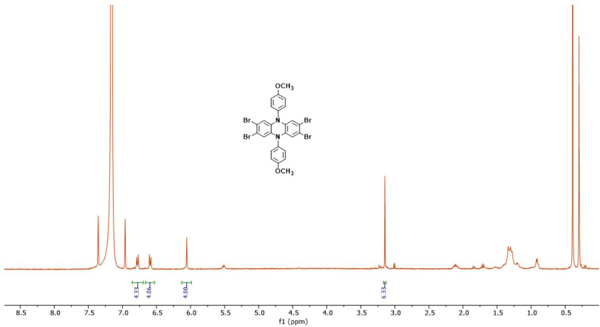
**Figure S115.**  $^1\text{H}$ -NMR spectrum of unpurified 4-4Br in  $\text{C}_6\text{D}_6$ .
