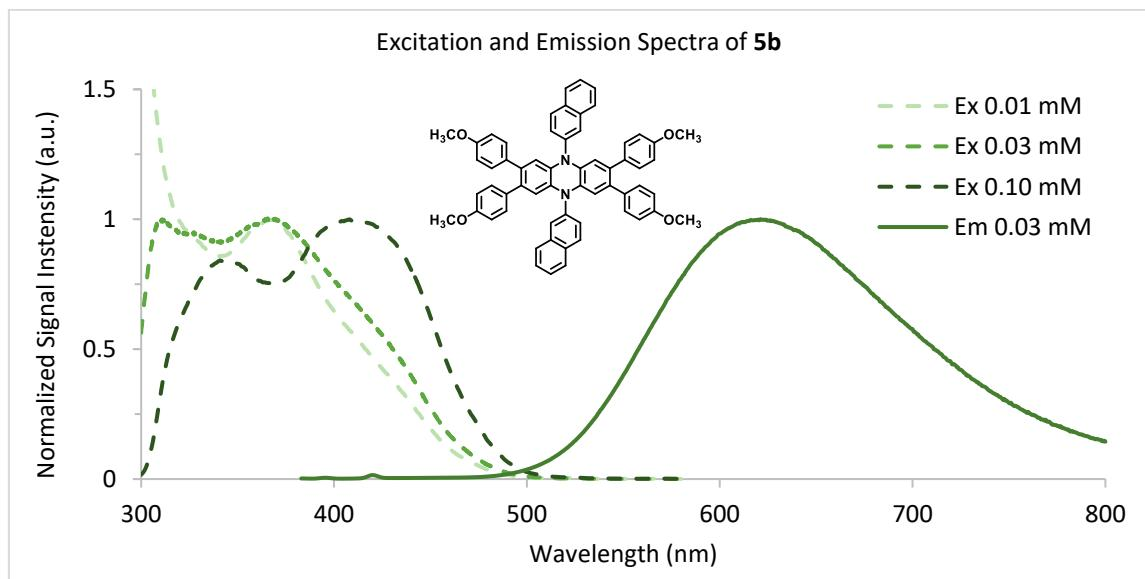
**Figure S17.** Fluorescence spectra of PC **5b**. Dashed lines are the excitation spectra at varying concentrations in DMAc and the solid line is the emission spectrum at 0.03 mM in DMAc. Emission spectra was collected using an excitation wavelength of 371 nm and is representative of emission profiles at all concentrations between 0.01 mM and 0.10 mM. Excitation spectra were collected for emission at 621 nm.
