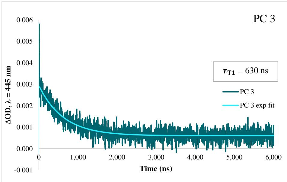
**Figure S36.** Kinetic absorption trace for PC 3 in DMAc at 445 nm with an exponential tail fit for determination of  $\tau_{\text{T1}}$ .
