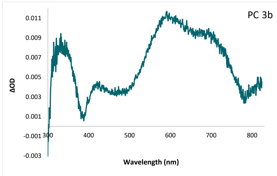
**Figure S21.** Spectral absorption of PC 3b in DMAc at a 200 ns time delay, with no emission subtraction. The ESA feature visible at  $\lambda = 593$  nm was followed by kinetic absorption. The spectral absorption data was offset corrected using kinetic data acquired at  $\lambda = 593$  nm.
