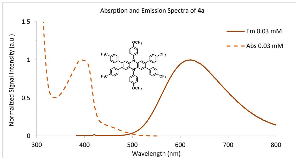
**Figure S14.** Emission spectra of PC **4a** (solid) and absorption spectra of **4a** (dashed) at 0.03 mM in DMAc. Absorption spectra was measured using UV-Vis and emission spectra was measured using fluorimetry. Emission spectra was collected using an excitation wavelength of 392 nm.
