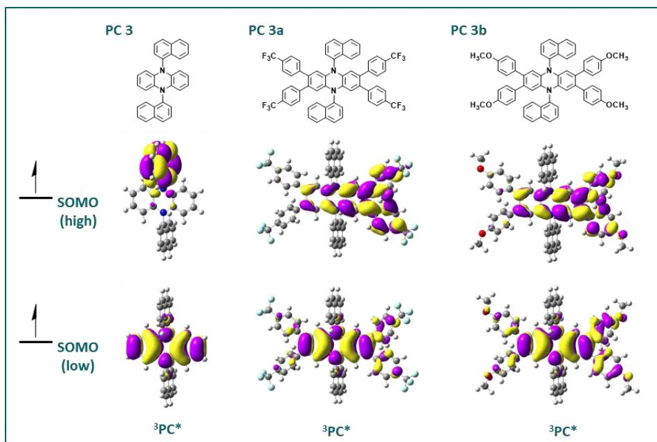
**Figure S70.** Computational modeling of the singularly occupied molecular orbitals (SOMOs) for PCs **3**, **3a**, and **3b** (from left to right); the lower lying SOMO (bottom row) and higher lying SOMO (top row) for each PC in the triplet excited state are shown.
