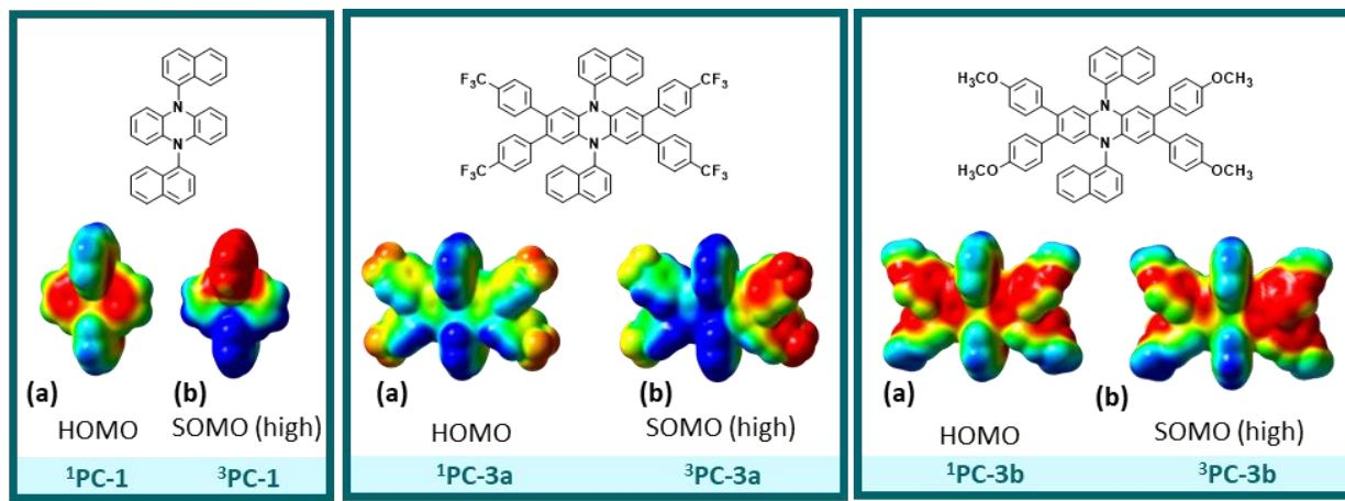
**Figure S73.** Electrostatic potential (ESP) mapped electron density for PCs **3**, **3a**, and **3b** (from left to right) in the ground state (a) and triplet excited state (b) are shown. Red color represents electron rich regions and blue color represents electron deficient regions.
