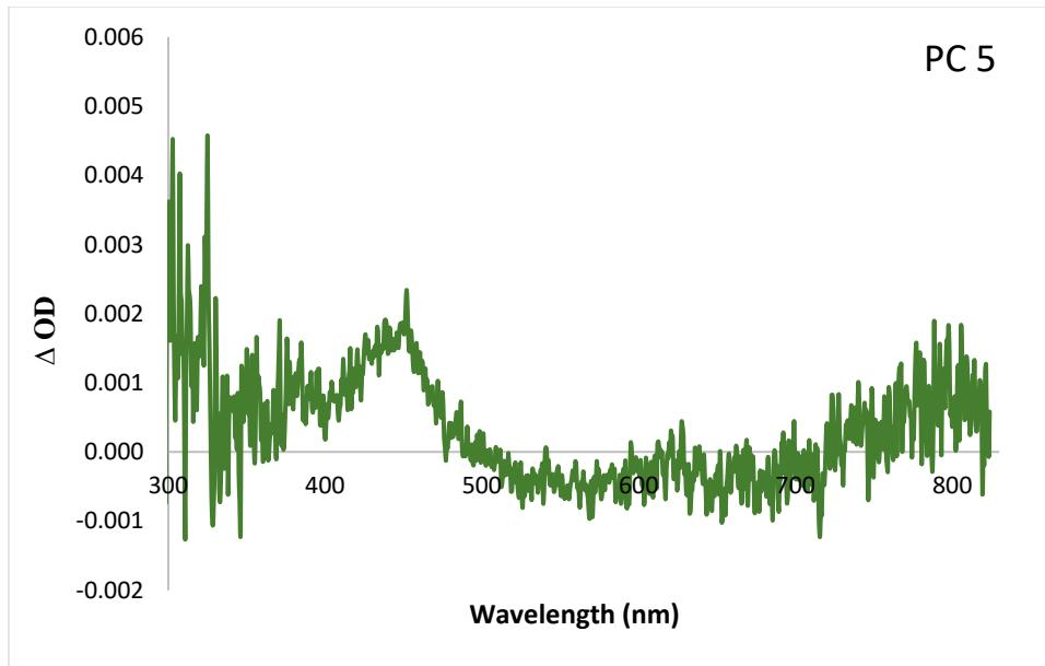
**Figure S25.** Spectral absorption of PC 5 in DMAc at a 200 ns time delay, with no emission subtraction. The ESA feature visible at  $\lambda = 450$  nm was followed by kinetic absorption. The spectral absorption data was offset corrected using kinetic data acquired at  $\lambda = 450$  nm.
