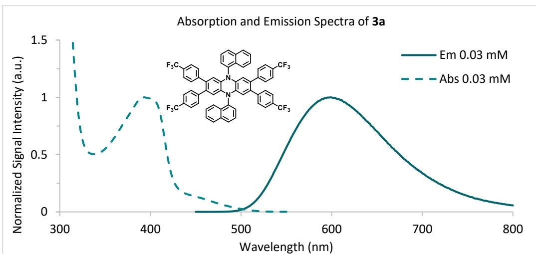
**Figure S10.** Emission spectra of PC **3a** (solid) and absorption spectra of **3a** (dashed) at 0.03 mM in DMAc. Absorption spectra was measured using UV-Vis and emission spectra was measured using fluorimetry. Emission spectra was collected using an excitation wavelength of 385 nm.
