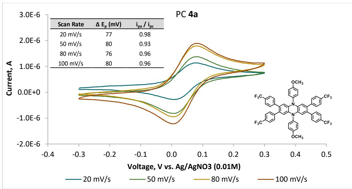
**Figure S58.** Cyclic voltammogram of PC 4a in DMAc at 20 mV/s, 50 mV/s, 80 mV/s, and 100 mV/s scan rates. Inserted into the graph is a chart showing the ratios of peak anodic current to peak cathodic current ( $i_{pa}/i_{pc}$ ) and the difference between peak anodic and peak cathodic current ( $\Delta E_p$ ) at each scan rate.
